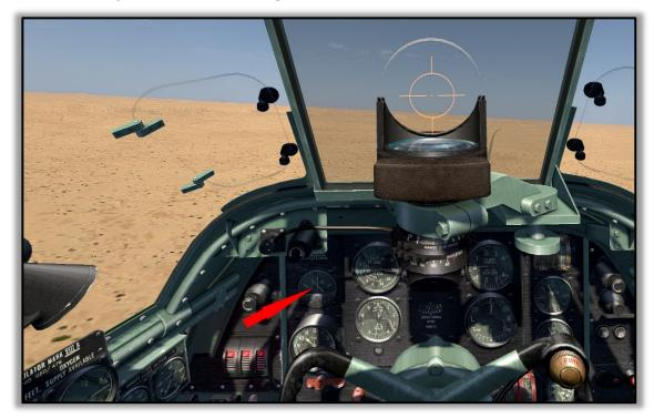
7) Turning the aircraft slowly to the left will gradually bring the 45-degree arms within the radio compass to line up with the 45-degree reference lines on each side of the centered vertical line. This indicates the aircraft is heading straight toward the homing beacon tower at the airfield.
