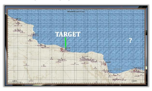
There are two radio beacons at Bardia and Sidi Barrani airfields. The first step is to use the radio compass to determine each beacon's deflection relative to your aircraft. Simply add those deflection headings to your current aircraft's course heading (270 degrees) which will give you the course heading you would need to fly to each. Draw a line to each, then use the reciprocal headings to show your location on the map where the two reciprocal lines intersect.
